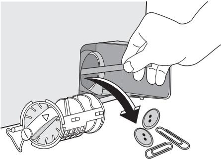
8. Check carefully whether the pump impeller rotates (it rotates jerkily). If it doesn't rotate, please contact your Service Centre.
